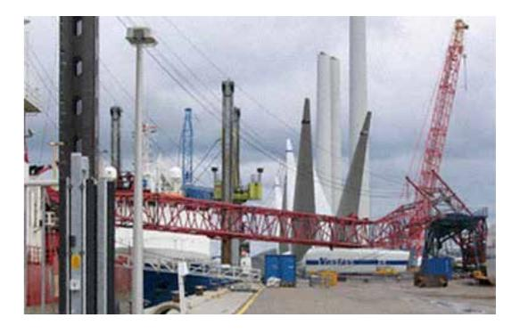
In the summer of 2007, an accident took place on the quayside of the ljmuiden port. The crane on an offshore installation barge fell on the quay and crashed. There was only limited damage to the wind turbine components; however, the crane itself could not be repaired anymore.
