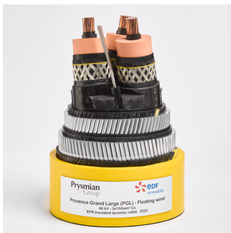
Figure 10. Model of 66 kV dynamic inter-array cable for the Provence Grand Large wind farm. Source: Prysmian, EDF Renouvelables.
